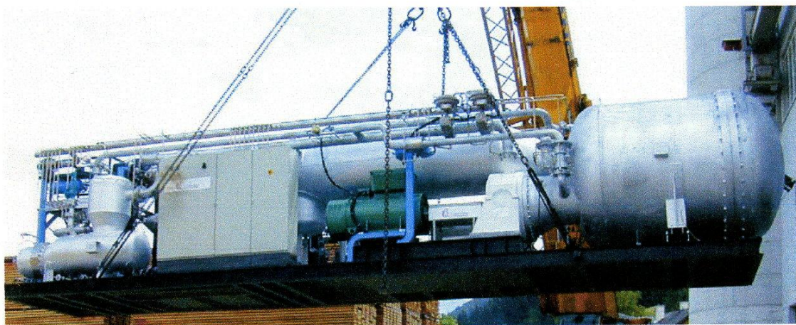
400 kW e ORC unit – EU demonstration project in Admont, Austria (Source: BIOS Bioenergy Systems, Austria, TURBODEN Srl, Italy, 2003)
